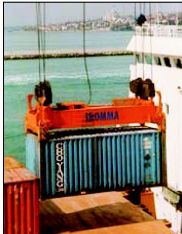
Figure 10.1: Spreader (hanging in a crane) for handling a single container.
