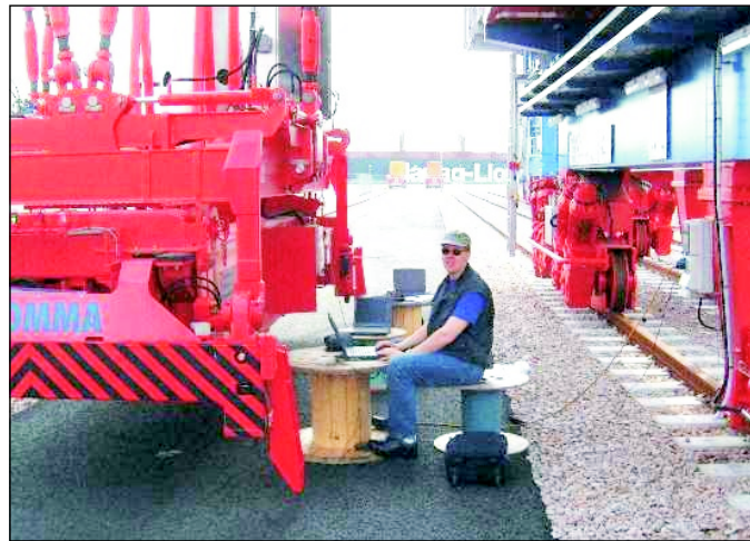
Figure 10.2: Spreader (left) standing on the ground under the crane (right). Containership at quay (background). Author downloading the controller software (middle).
